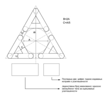
Size of the marking shall be determined by the vertical dimension B of the marking which may only have values of standard numbers rounded up, to the order of
