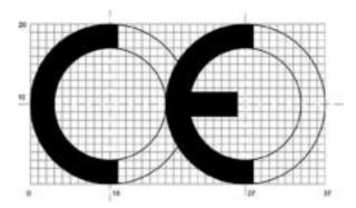
The vertical dimension of the CE marking shall, as a rule, be at least 5 mm. If the CE marking is reduced or enlarged, the proportions given in the above graduated drawing must be respected.
